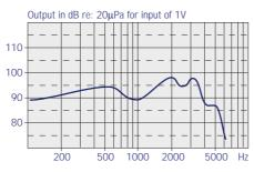
Total harmonic distortion: typically 15% at 1kHz (drive=10mW) (headset measured on a B&K artificial ear with flat plate coupler) Intelligibility: Speech Transmission Index STI>0.78
